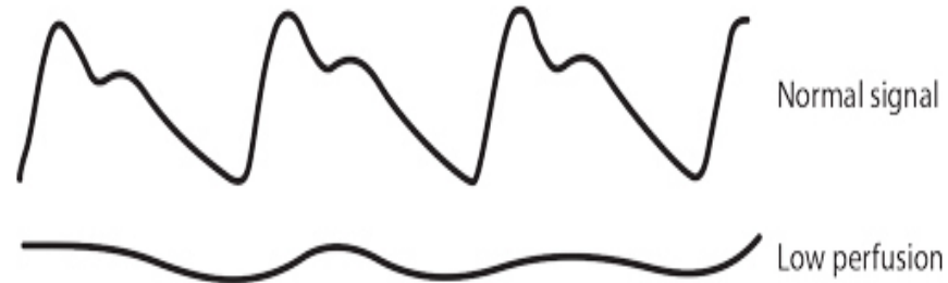
Figure 4: Normal vs. low perfusion pleth waveforms
